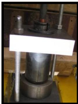
Figure 3 - CFRP anchor
