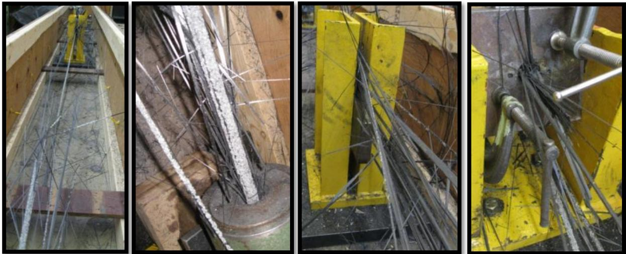
Figure 8 - Tendon rupture failures
