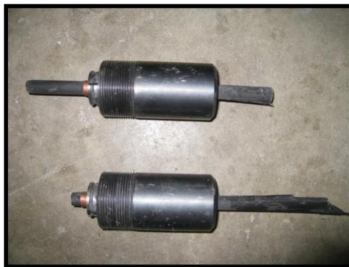
Figure 9 - Tendon anchors after failure
