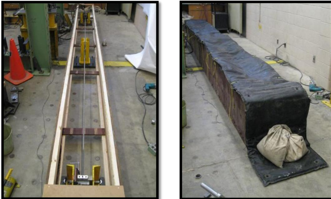
Figure 2 - a) Test setup, and b) Protective box and removable blanket
