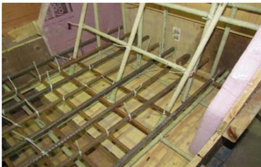
Fig. 5 View of GFRP bars in Model 1
