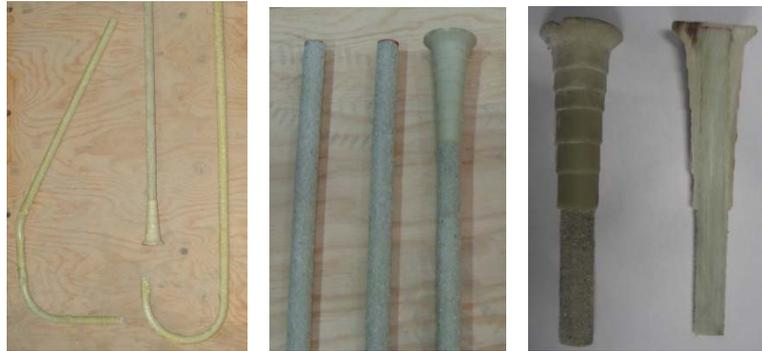
Fig. 2 View of GFRP bars types
