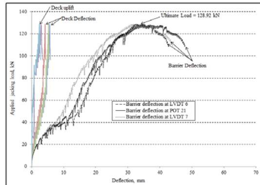
Fig. 22 Load-deformation curve of the barrier wall, deck movement and deck uplift of barrier model 5
