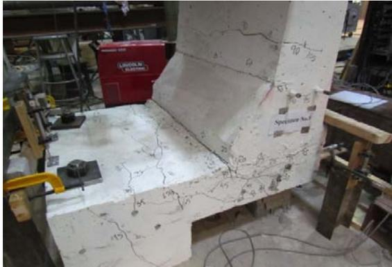
Fig. 21 View of the crack pattern in barrier model 5 with steel bars at 200 mm spacing
