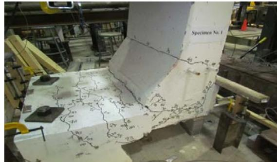
Fig. 12 View of the crack pattern in barrier model 1 with HM-GFRP bars at 300-mm spacing (right side)
