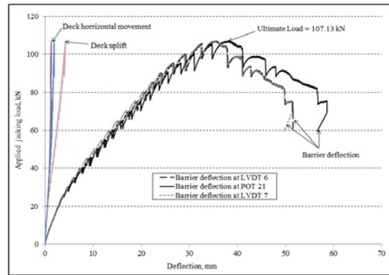
Fig. 18 Load-deformation curve of the barrier wall, deck movement and deck uplift of barrier model 3
