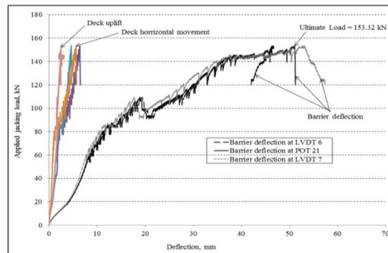
Fig. 20 Load-deformation curves of the barrier wall, deck movement and deck uplift of model 4
