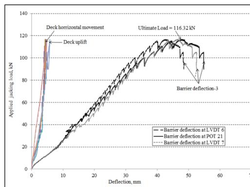
Fig. 16 Load-deformation curve of the barrier wall, deck movement and deck uplift of barrier model 2
