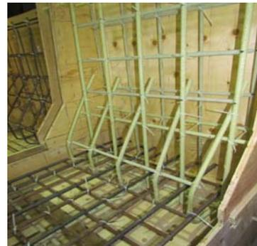
Fig. 6 View of GFRP bars in Model 2
