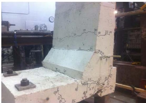
Fig. 15 View of the crack pattern in barrier model 2 with SM-GFRP bent bars at 200 mm spacing
