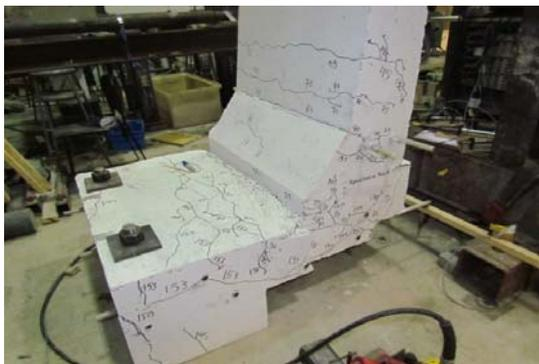
Fig. 19 View of the crack pattern in barrier model 4 with HM-GFRP bars at 150 mm spacing
