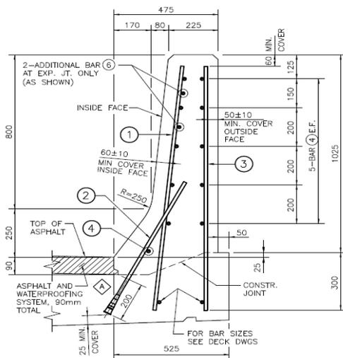
Fig. 3a Barrier detailing from MTO Standard Drawing SS110-92 (MTO, May 2011)
