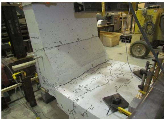
Fig. 13 View of the crack pattern in barrier model 1 with HM-GFRP bars at 300-mm spacing (left side)
