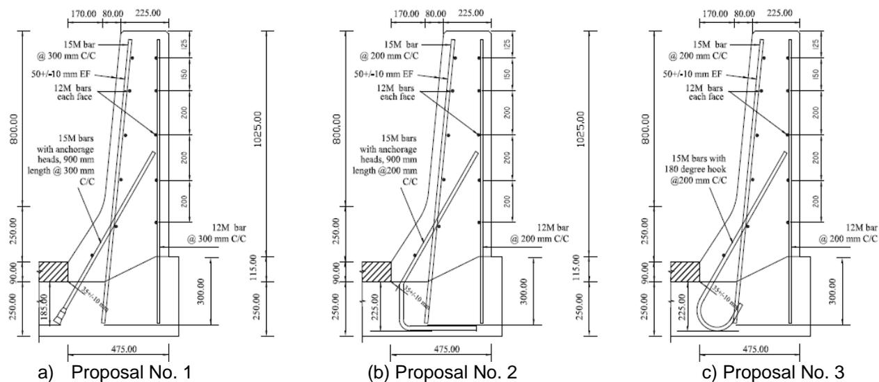
Fig. 4 Proposed Ryerson University GFRP-Reinforced Barrier Details
