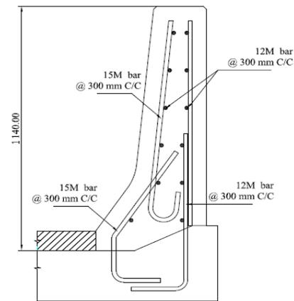
Fig. 3b Traditional barrier reinforcement with bent bars
