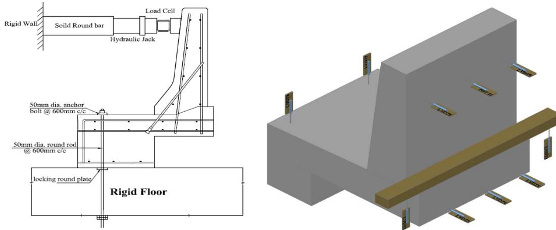
Fig. 10 Schematic diagram of test setup (left) and locations of LVDT's (right)
