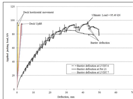
Fig. 14 Load-deformation curves of the barrier wall, deck movement and deck uplift of barrier model 1
