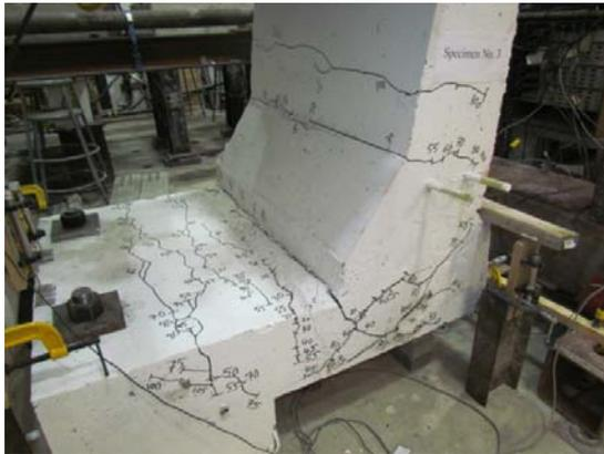
Fig. 17 View of the crack pattern in model 3 with SM-GFRP bars with 180° hooks at 200 mm spacing
