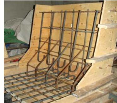
Fig. 9 View of barrier model 5
